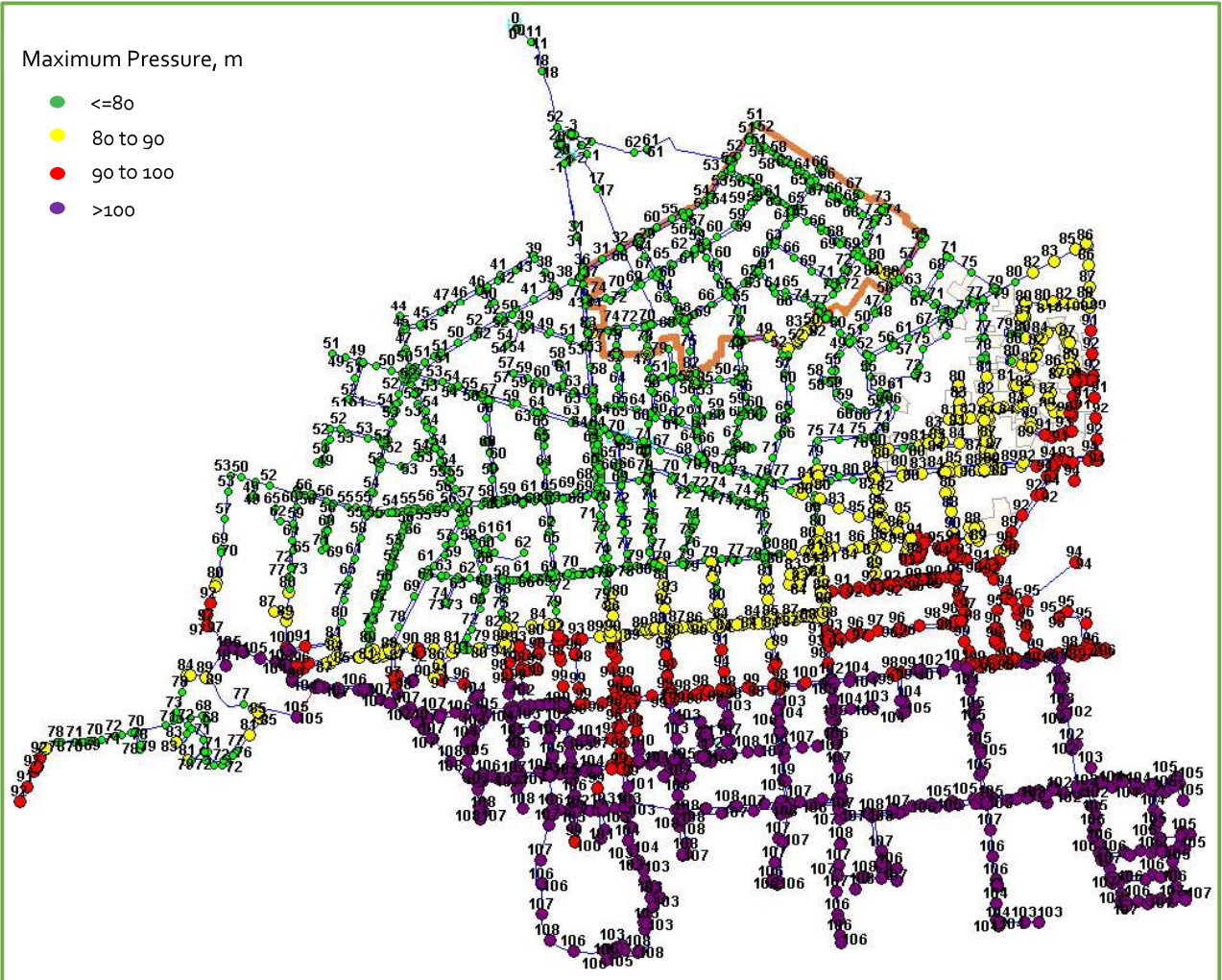
Figure 8: Onehunga Water Network Maximum Pressures
